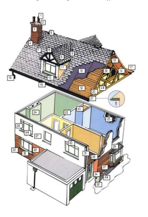
14 Trusses 15 Collar 16 Insulation 17 Parapet gutter 18 Eaves guttering 19 Rainwater downpipe 20 Verge boards / skews 21 Soffit boards 22 Partition wall 23 Lath / plaster 24 Chimney breast 25 Window pointing 26 Window sills 27 Rendering 28 Brickwork / pointing 29 Bay window 30 Lintels 31 Cavity walls / wall ties 32 Subfloor ventilator 33 Damp proof course 34 Base course
