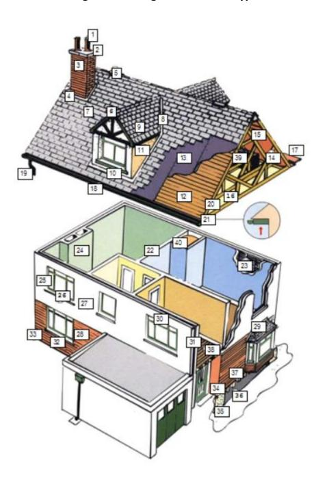
Valley guttering Dormer projection 10 Dormer flashing 11 Dormer cheeks 12 Sarking 13 Roof felt 14 Trusses 15 Collar 16 Insulation 17 Parapet gutter 18 Eaves guttering 19 Rainwater downpipe 20 Verge boards / skews 21 Soffit boards 22 Partition wall 23 Lath / plaster 24 Chimney breast 25 Window pointing 26 Window sills 27 Rendering 28 Brickwork / pointing 29 Bay window 30 Lintels 31 Cavity walls / wall ties 32 Subfloor ventilator 33 Damp proof course 34 Base course 35 **Foundations**
